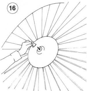
Insert COVER CONE over carriage bolt in center of support disc, place washer over bolt and fasten down with top PYRAMID FINIAL as illustrated.
