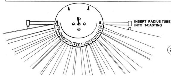
8 Insert ends of radius tube (extending from each side of umbrella section) into T-Casting support arms.
