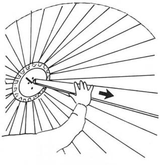
Place the two UMBRELLA TOP PANS over the openings between the two umbrella sections as illustrated. The hole at the narrow end of the umbrella top pan fits over the stud on support disc where both umbrella sections meet. Secure with #10-24 hex nut and tighten all nuts to studs at this time.
